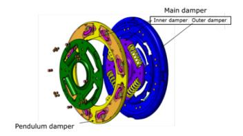
Fig. 11 Pendulum vibration damper
