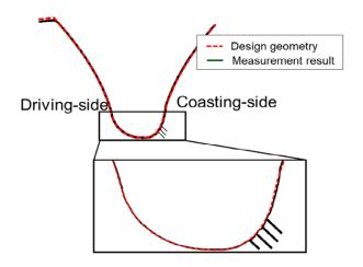
Fig. 9 Comparison of calculated and measured geometries
