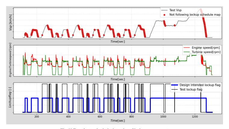
Fig. 11 Function to check the intention of lockup engagement
