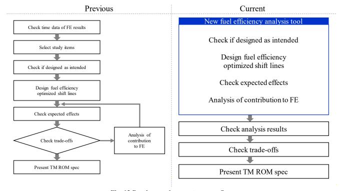
Fig. 12 Previous and current process flow
