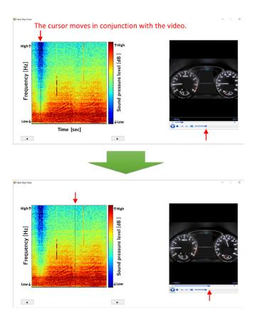
Fig. 5 Movement of spectrogram cursor linked to video of vehicle instruments
