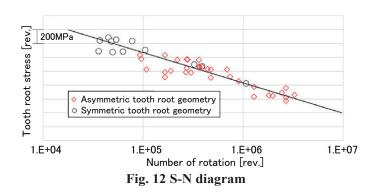
It is seen that the test results for both the symmetric and asymmetric tooth root geometries are plotted on the same S-N curve. Consequently, the results confirm that the method proposed for calculating tooth root stress is also applicable to gears having an asymmetric tooth root radius of curvature.
