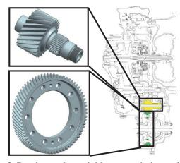
Fig. 2 Continuously variable transmission unit for medium to large passenger cars and a second reduction gear pair.
