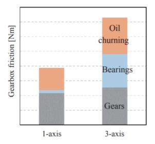
Fig. 10 Gearbox friction loss
