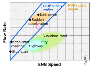
Fig. 5 Twin oil pump system concept
