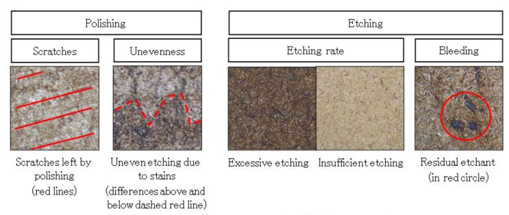
Fig. 3 Typical uncertain elements at the time of specimen preparation
