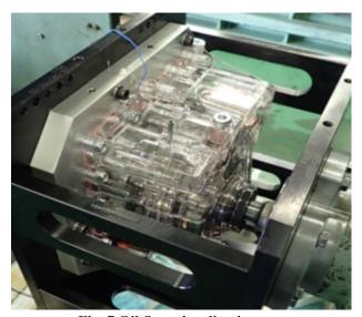
Fig. 7 Oil flow visualization test
