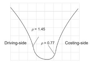
Fig. 6 Tooth root geometry
