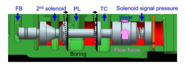
Fig. 8 Control valve (pressure regulator valve)
