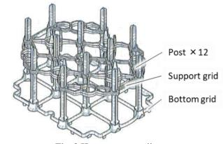
Fig. 2 Heat treatment jig
