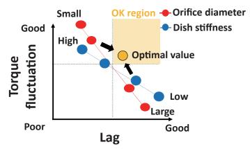
Fig. 8 Optimal design for selector lever performance
