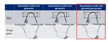
Fig. 4 Comparison of hob and workpiece
