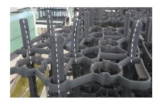
Fig. 5 Heat treatment jig
