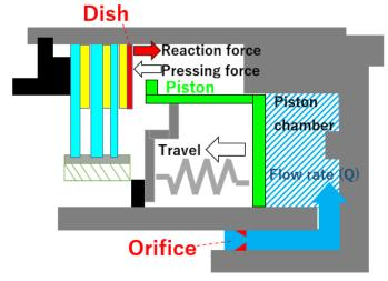
Fig. 7 Configuration of forward/reverse changeover system
