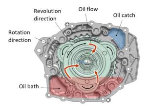
Fig. 3 Oil flow under low speed
