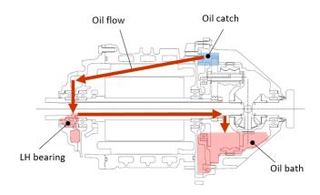
Fig. 5 Oil flow for LH bearing
