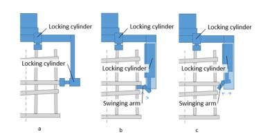
Fig. 12 Clamping method
