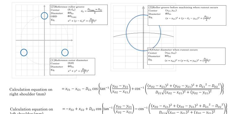
Fig. 5 Calculation equation for machining allowance on right/left shoulders and relate elements
