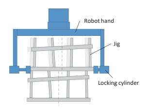
Fig. 11 Clamping system using a locking cylinder
