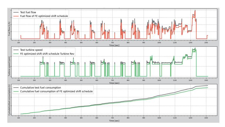
Fig. 10 Function to compare test results and FE optimized shift schedule
