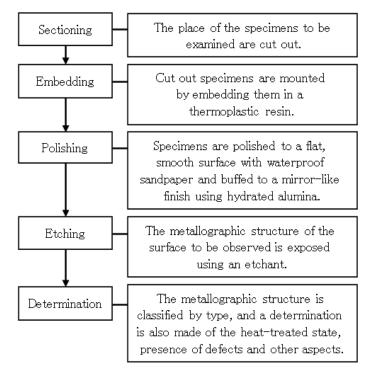
Fig. 1 Metallographic examination procedure and descriptions
