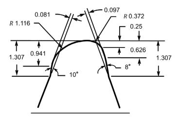
Fig. 5 The specific tool dimensions
