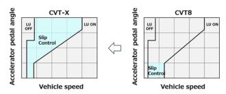
Fig. 10 Slip control region at vehicle launch
