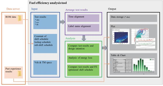
Fig. 5 Flowchart of inputs & outputs
