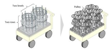
Fig. 3 Heat treatment jig trolley
