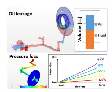
Fig. 5 Characteristics obtained by 3D CFD simulation
