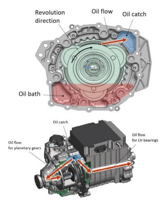
Fig. 2 Lubrication system for 1-axis e-Axle
