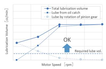
Fig. 8 Results of planetary gear lubrication volume measurement
