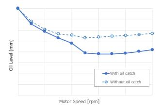
Fig. 9 Results of gearbox oil level measurement
