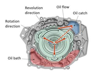
Fig. 4 Oil flow under high speed
