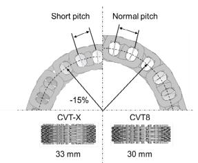
Fig. 4 Pitch comparison for previous and new chains
