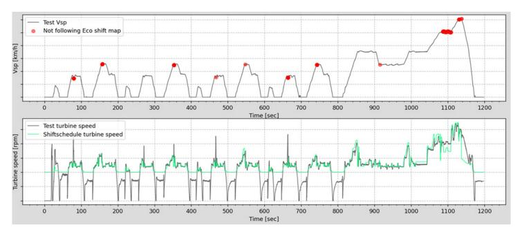
Fig. 9 Function to check the intention of shift schedule
