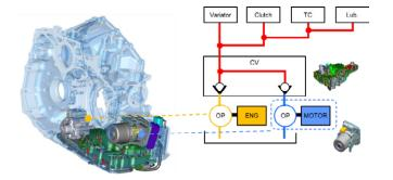
Fig. 6 Twin oil pump system layout
