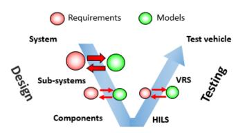
Fig. 1 Model application to V-shaped development process
