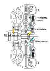
Fig. 9 3-way oil flow route of torque converter
