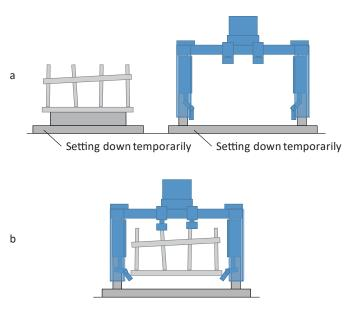
Fig. 14 Specification for temporarily setting down heat treatment jig
