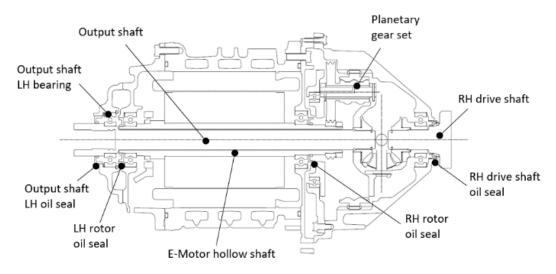
Fig. 1 1-axis e-Axle structure
