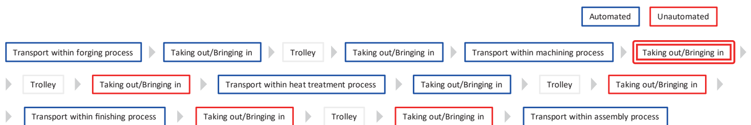
Fig. 1 Pulley production line processes
