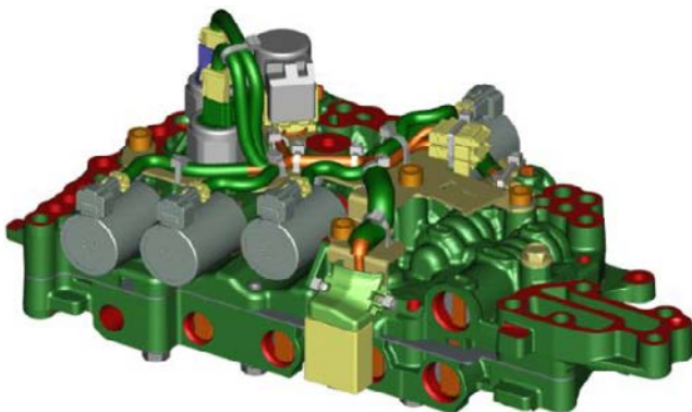
Fig. 1 Structure of control valve
