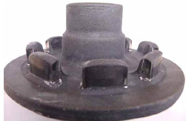
Fig. 12 Parking gear underfill defect
