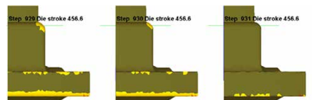
Fig. 14 Simulation results following addition of protrusion to finishing die
