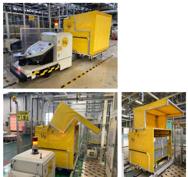
Fig. 3 Gull-wing structure for automatically opening/closing the cargo door
