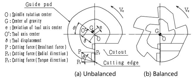
Fig. 13 Cross section of reamer
