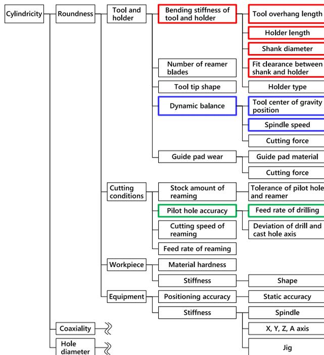
Fig. 4 Cause and effect diagram for improving cylindricity
