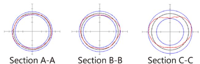
Fig. 3 Roundness profile of reamed spool hole
