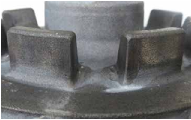
Fig. 15 Parking gear after addition of small protrusion
