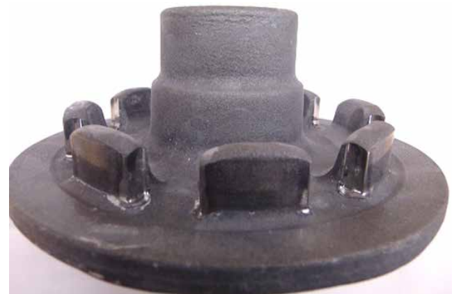
Fig. 12 Parking gear underfill defect
