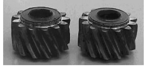
Fig.2 Planetary pinion gear by precision gear forging
