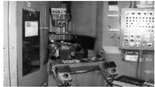
Fig.7 View of the old transfer machine by Kingsbury company, that are now working.
