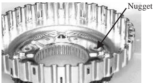
Fig.9 Example of projection welding in CVT parts
