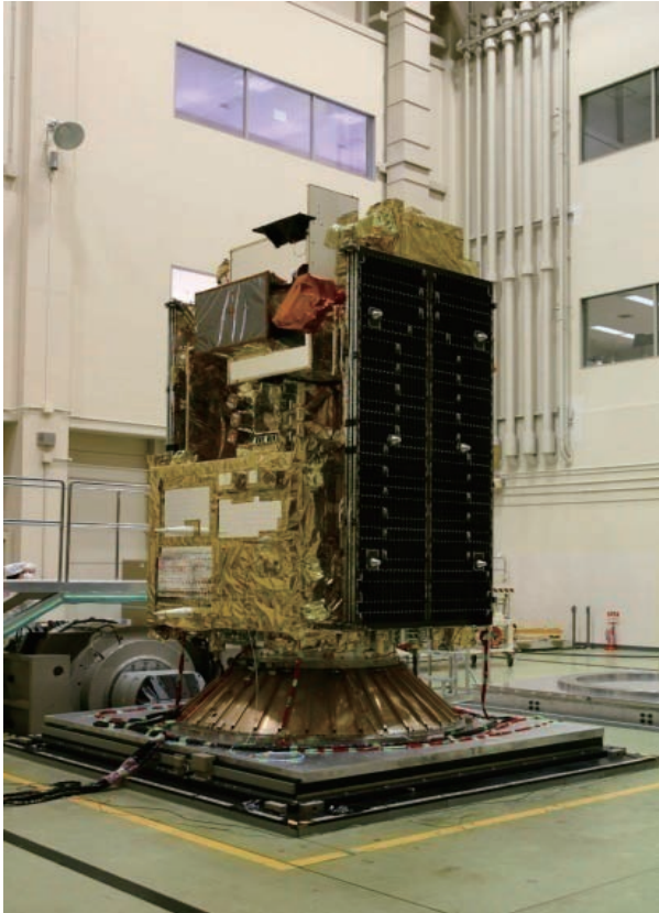
Fig. 6 Ibuki undergoing a vibration test at the JAXA Tsukuba Space Center
