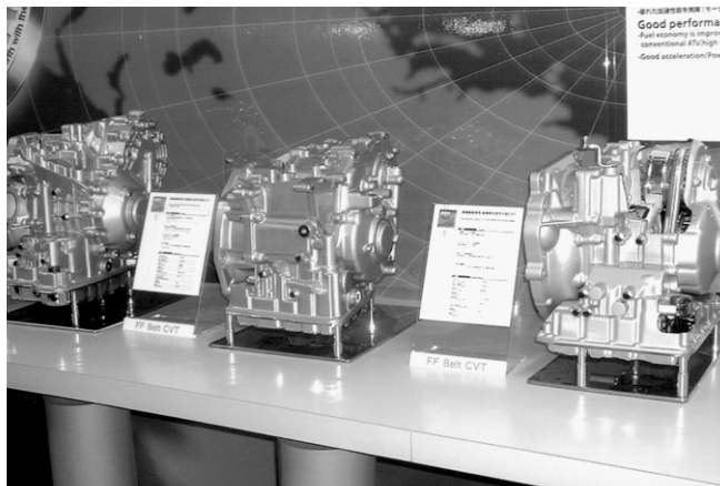
Fig. 9 Next-generation Belt CVTs
