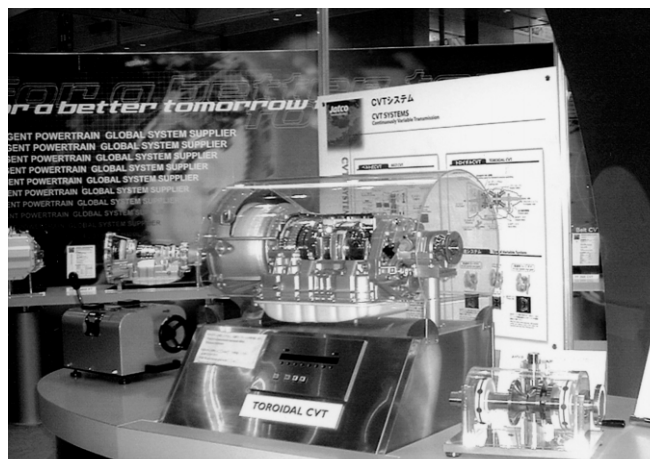
Fig. 6 Cutaway model of toroidal CVT
