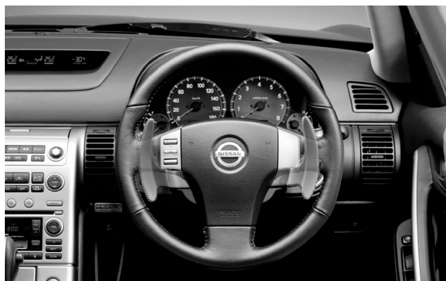
Fig. 2 Paddle shifter mounted behind the steering wheel (The photo was processed by computer to show a see-through view of the paddles.)
