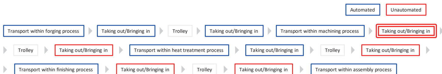
Fig. 1 Pulley production line processes
