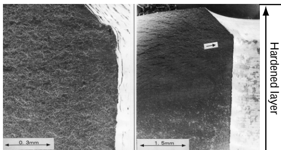
b) The crack grew from hardened layer (Effective case depth : 4.0mm)
