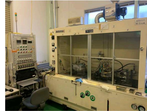
Fig. 4 Previous control valve tester
