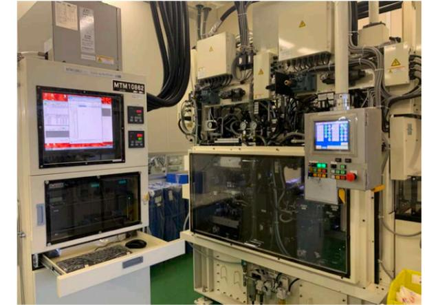
Fig. 5 New control valve tester
