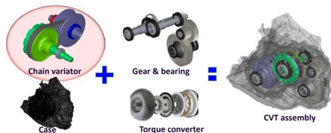
Fig. 14 Configuration of integrated CVT system
