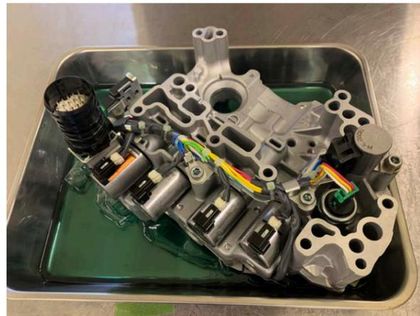
Fig. 3 Example of control valve assembly
