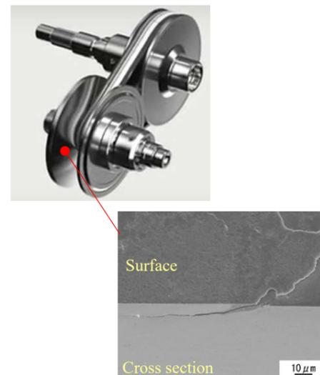
Fig. 3 Peeling wear on pulley sheave
