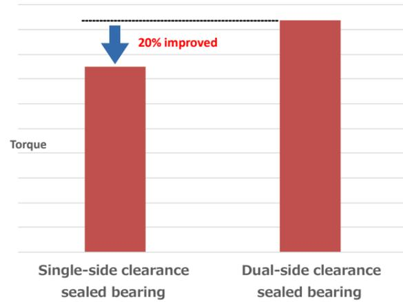
Fig. 6 Results of friction measurement
