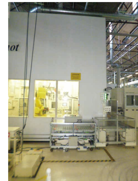
Fig. 8 MS peening machine in negative pressure room
