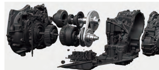
Fig. 1 CVT internal structure model
