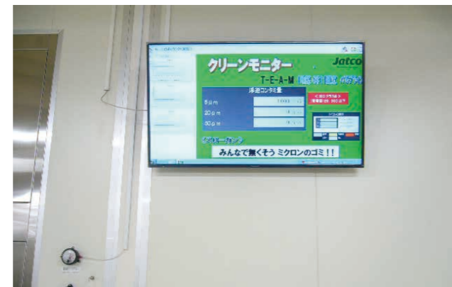
Fig. 6 Particle counter and TV monitor
