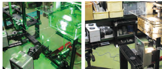
Fig. 5 Camera arrangement (left) PIV and (right) stereopsis
