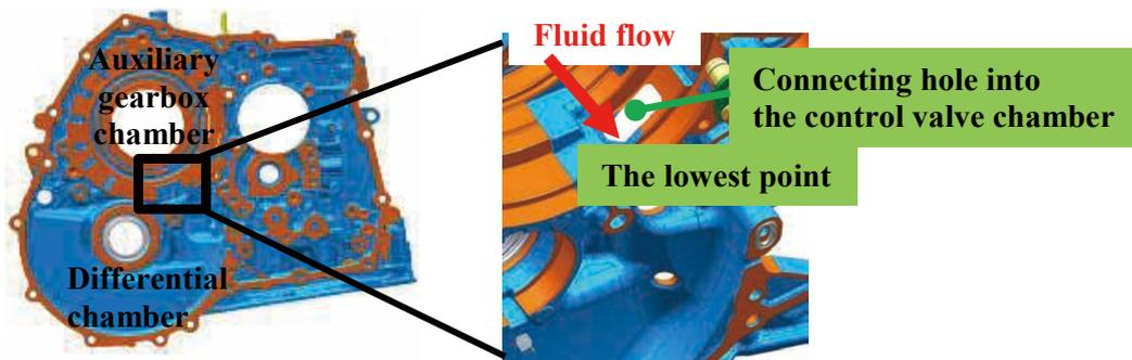
Fig. 5 Optimized shape of auxiliary gearbox case
