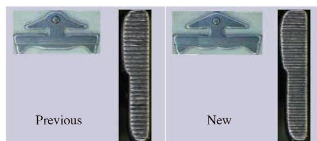
Fig. 1 Newly developed 24-mm belt
