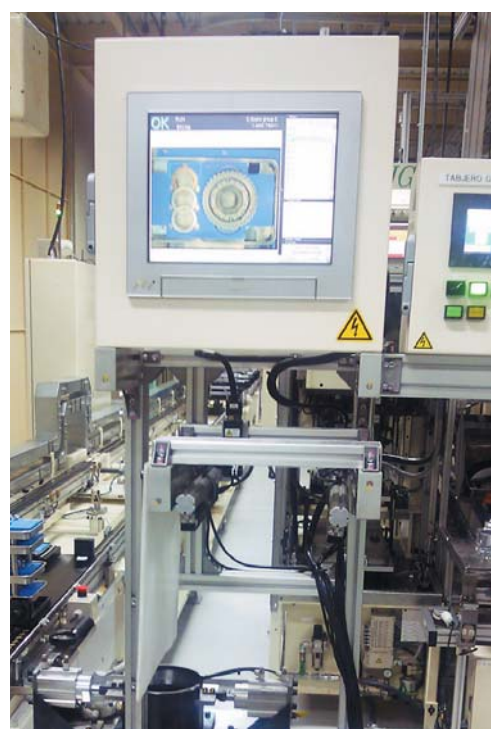
Fig.9 Pokayoke by image processing system
