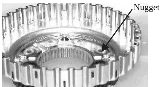
Fig.9 Example of projection welding in CVT parts
