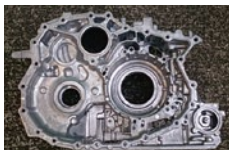
Transmission case with reduced wall thickness
