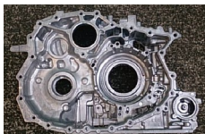
Transmission case with reduced wall thickness
