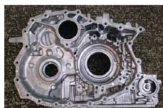
Transmission case with reduced wall thickness
