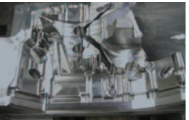
Die-cast mold, produced through a direct carving process
