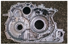
Transmission case with reduced wall thickness
