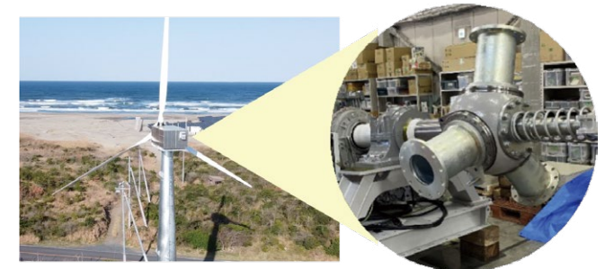
Power generation gearbox (nacelle)
