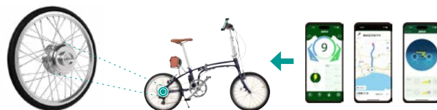
Drive unit integrating assist motor and transmission mechanism
