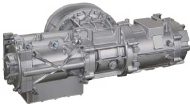
e-Axle (with multi-speed transmission)
