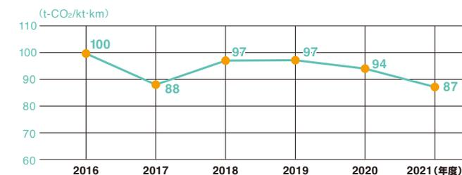
\*CO<sub>2</sub>排出量原単位: CO<sub>2</sub>排出量(t-CO<sub>2</sub>)÷輸送荷量(kt-km)
