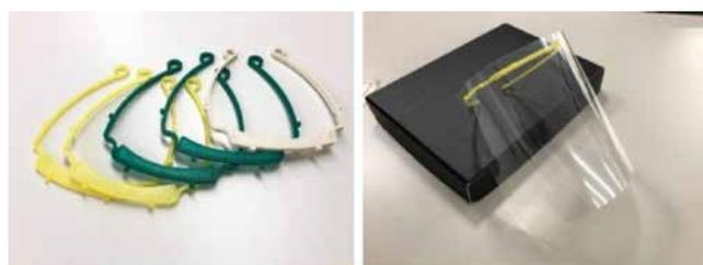
Frames produced with a 3D printer
