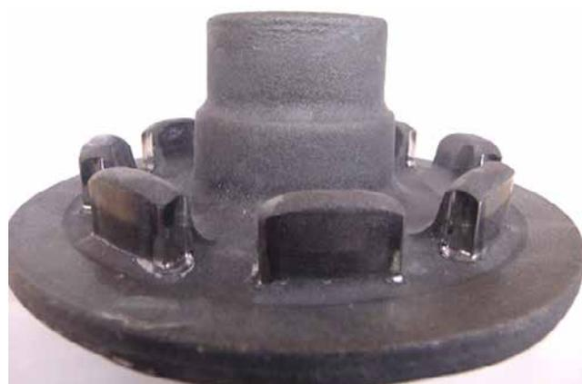
Fig. 12 Parking gear underfill defect
