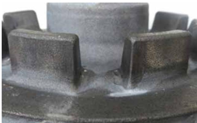
Fig. 15 Parking gear after addition of small protrusion
