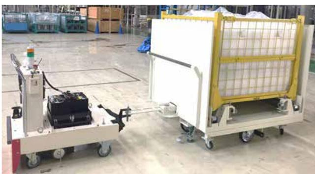
Fig. 1 Towing type AGV
