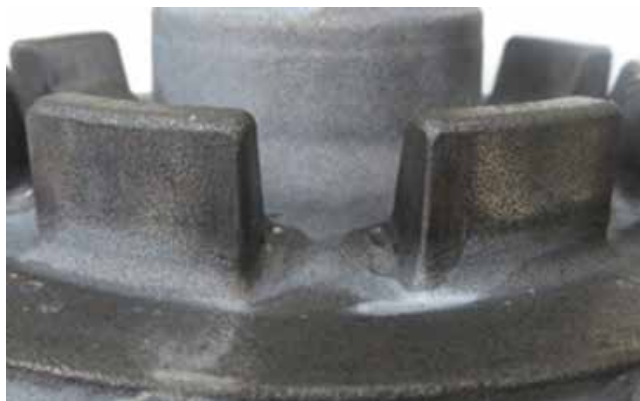
Fig. 15 Parking gear after addition of small protrusion
