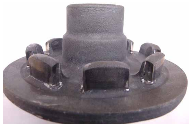
Fig. 12 Parking gear underfill defect
